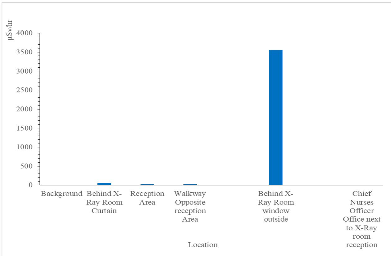
Figure 8: Radiological facility H Radiation Dose rate at different locations
